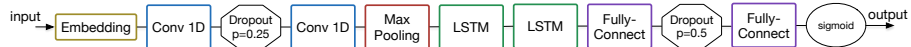
Fig. 12: Network Architecture We use an 8 layer deep learning model. It is primarily built around the LSTM layers, which develop the temporal relationships between instructions. The CNN layers vastly increase the stability of the model while also aiding in preventing it from overfitting. The DNN layers at the end bring everything from the previous layers together in a classification value stating if it was given matching function representations.
