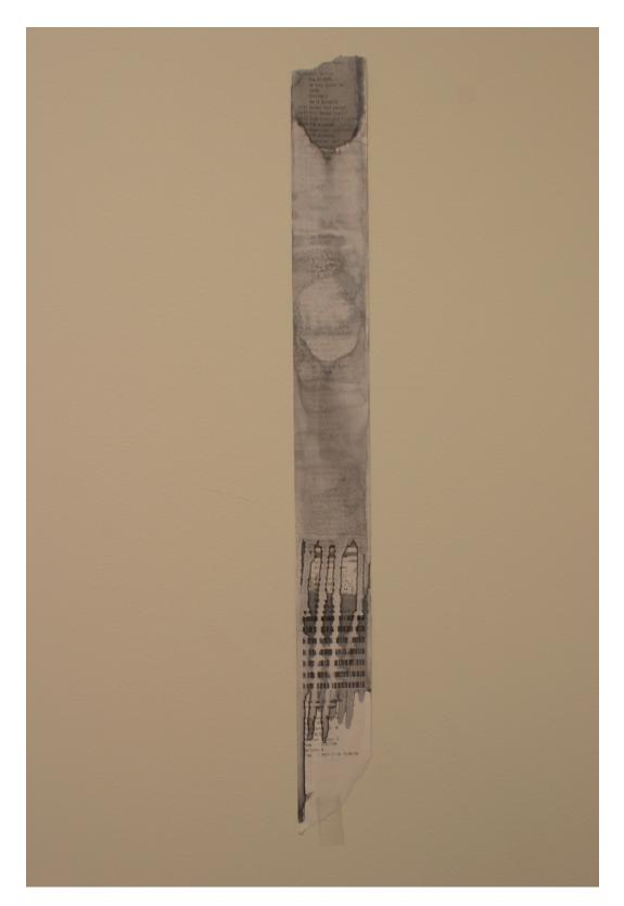
Figure 14.3: A paper copy of the system log destroyed by injecting a household chemical into the AV-TSX. No seals were broken in this attack.
