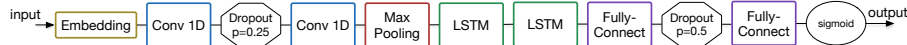
Fig. 12: Network Architecture We use an 8 layer deep learning model. It is primarily built around the LSTM layers, which develop the temporal relationships between instructions. The CNN layers vastly increase the stability of the model while also aiding in preventing it from overfitting. The DNN layers at the end bring everything from the previous layers together in a classification value stating if it was given matching function representations.
