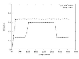
Figure 12: Channel utilization under SRP
