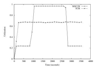
Figure 16: Channel utilization under DCA
