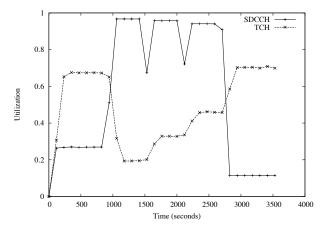
Figure 14: Channel utilization under DRP
