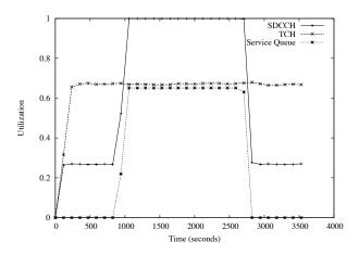
Figure 8: The simulated utilization for a sector implementing WFQ. Notice that TCH utilization remains constant throughout the attack.
