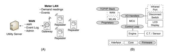
Figure 1: Smart meter operation. Figure (a) shows the two tiered structure of meter-utility communications. Figure (b) shows a typical smart meter architecture.
