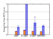
(b) The average RTT (*ms*) of **ping** command without target binding in the ARP cache for 1000 ICMP echo requests over 10 runs. The right bar is the average RTT of the first **ping** during the 10 runs.
