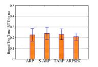
(a) The average RTT (ms) of ping command with the target binding in the ARP cache for 1000 ICMP echo requests.
