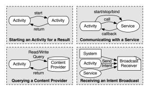
Figure 2: Typical IPC between application components
