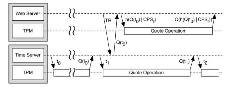
Fig. 5. Server quote generation - The server requests the most recent timestamp from the time server (Q(t<sub>0</sub>)), and then generates a quote using the most recent hash tree computed ( $CPS_r$ ).
