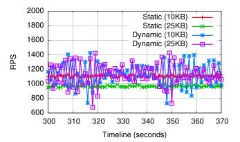
Fig. 10. Integrity measured web server throughput – sustained RPS during a 70 second experiment.
