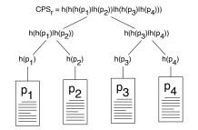
Fig. 4. A Merkle hash tree base for the cryptographic proof system. The leaf nodes are hashes of the pages served to clients.
