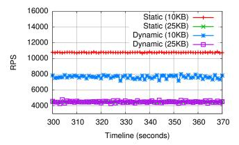
Fig. 9. Unaltered web server throughput – sustained RPS during a 70 second experiment.
