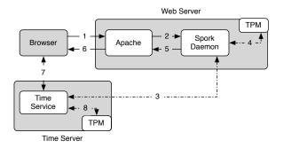
Fig. 8. An overview of the Spork system architecture – The time server provides an attested timestamp to the web server which is bound to the content delivered to the browser and local software integrity information.
