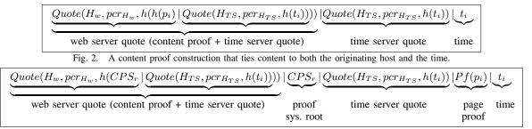
Fig. 3. Extended content proof that uses a cryptographic proof system as the challenge rather than a document hash. A succinct page proof is also included.
